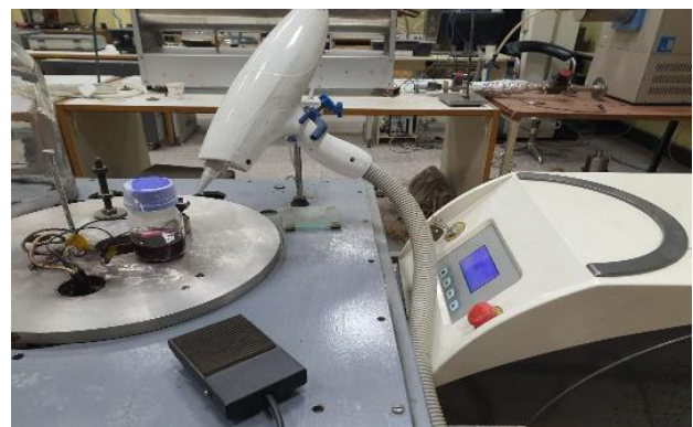
Figure 2. PLD device used in preparation of CoFe_2O_4 .
