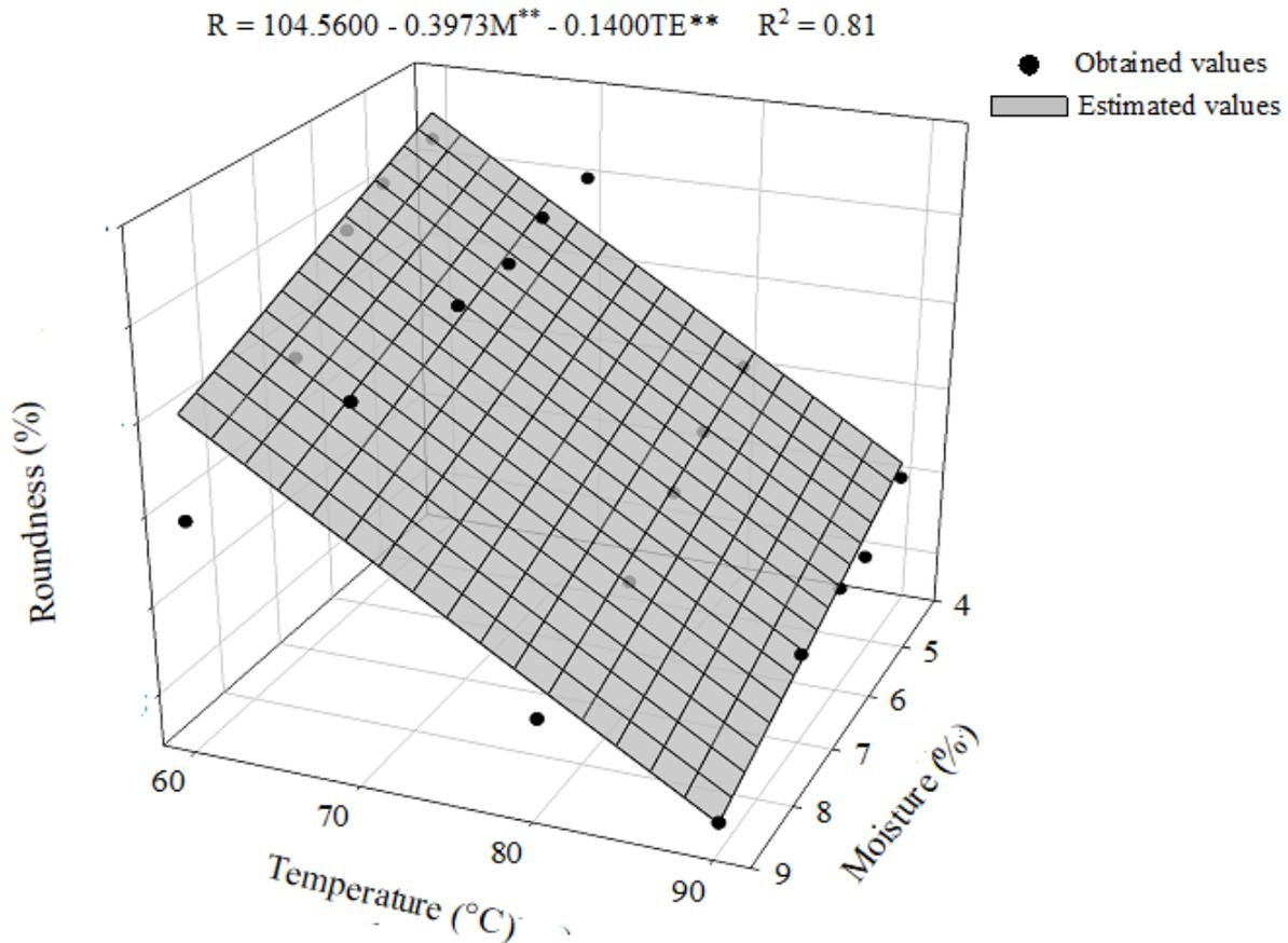
**Figure 3.** Roundness (%) of macauba fruit kernels as a function of moisture and temperature. \*\* Significant at 1% by the t-test.
