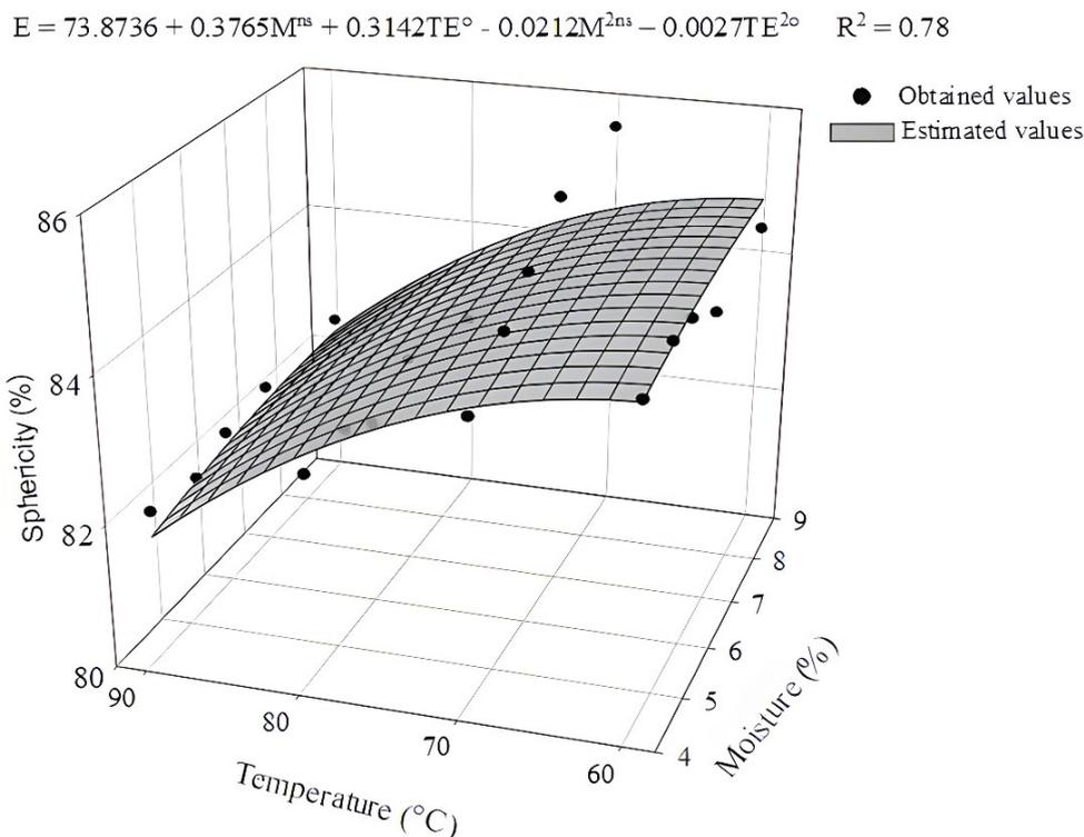
**Figure 2.** Sphericity (%) of macauba fruit kernels as a function of moisture and temperature. ° Significant at 10% and <sup>ns</sup> Not significant by the t-test.
