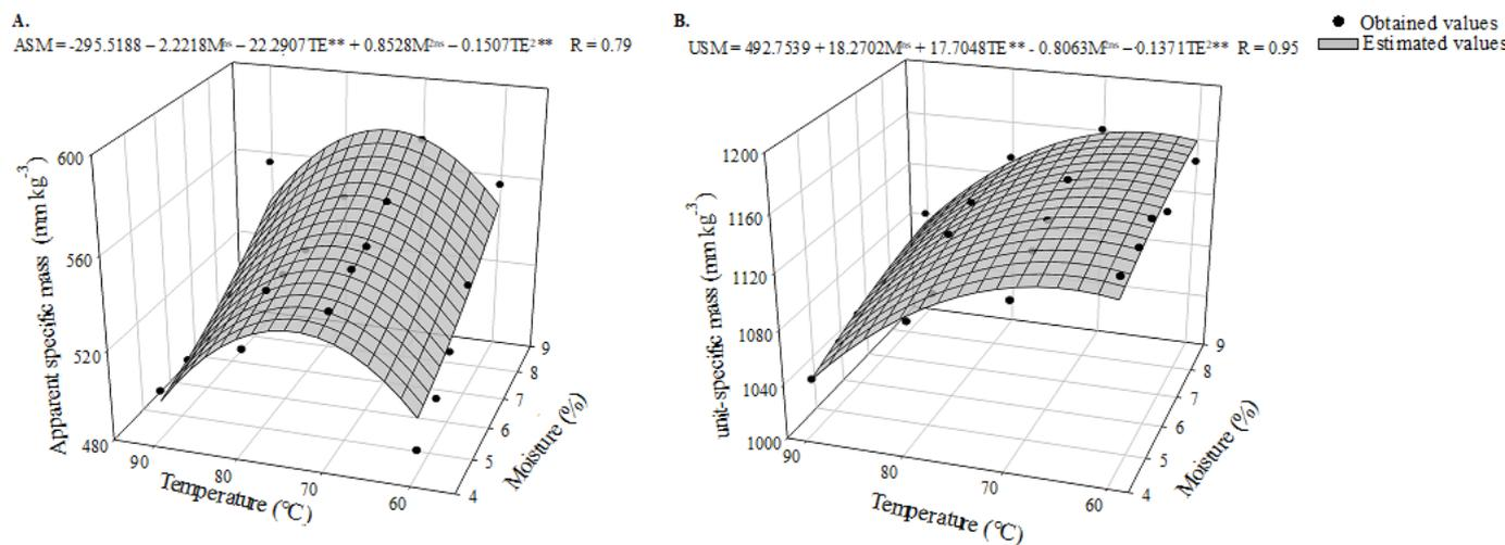
**Figure 5.** Apparent specific mass (A) and unit-specific mass (B) of macauba fruit kernels as a function of moisture and temperature. \*\* Significant at 1% and <sup>ns</sup> Not significant by the t-test.
