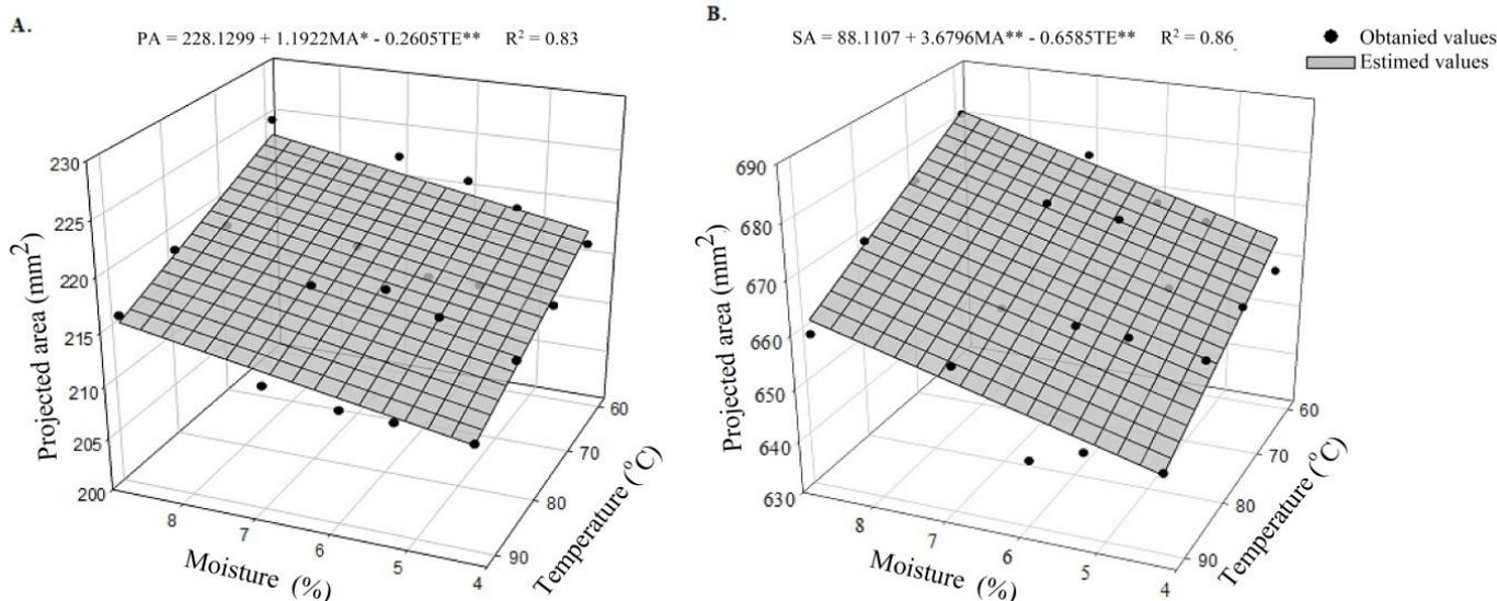
**Figure 4.** Projected area (A) and surface area (B) of macauba fruit kernels as a function of moisture and temperature. \* Significant at 5% and \*\* Significant at 1% by the t-test.
