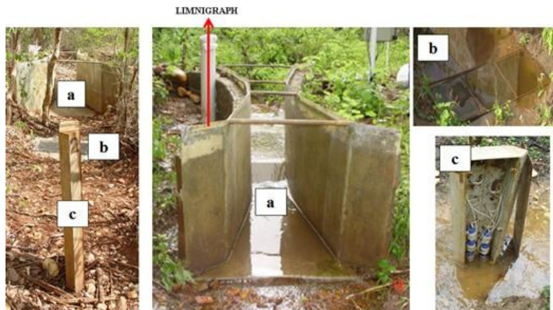
Figure 3. Parshall flume (a), pit to collect dragged sediment (b) and tower to collect suspended sediment (c) installed in each watershed of the Iguatu Experimental Basin.
