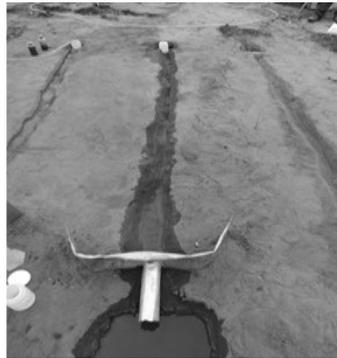
**Figure 2.** Preformed rill following the natural slope of the terrain, energy sinks buried at the upper end, and liquid and solid discharge collector installed at the lower end.
