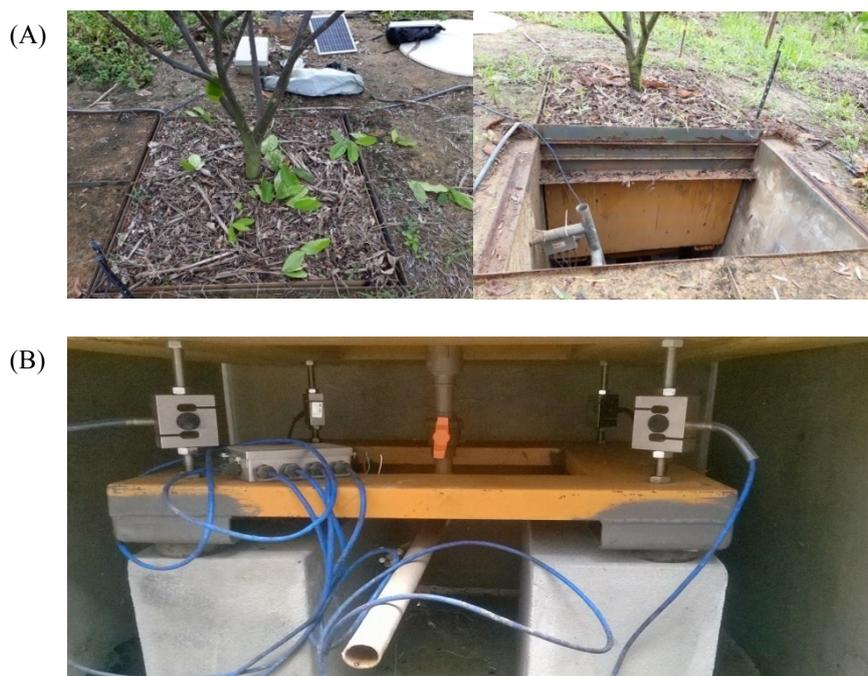
**Figure 1.** Cultivation of clonal cocoa - CCN 51 in a lysimeter box (A) installed on four load cells (B).
