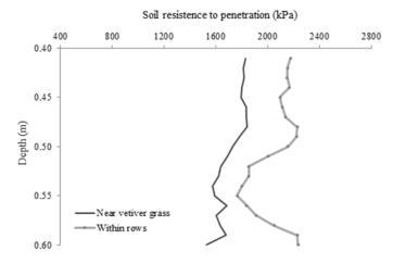
Figure 7. Mechanical resistance of the Neossolo Flúvico to penetration at 0.40–0.60 m depth, at points near the vetiver grass and at points within rows.
