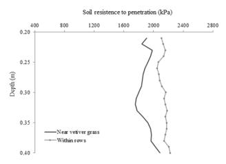
**Figure 6**. Mechanical resistance of the Neossolo Flúvico to penetration at a depth of 0.20–0.40 m, at points near to vetiver grass plant and at points within rows.
